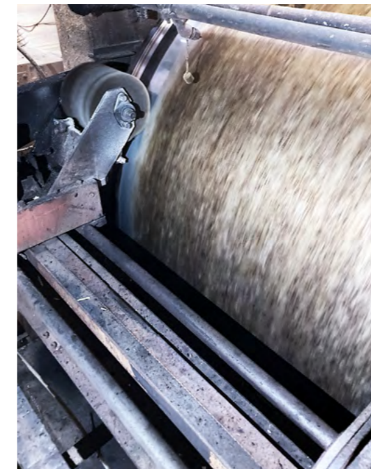
without impress products brown steel belt with adhesive flakes (bad function)
